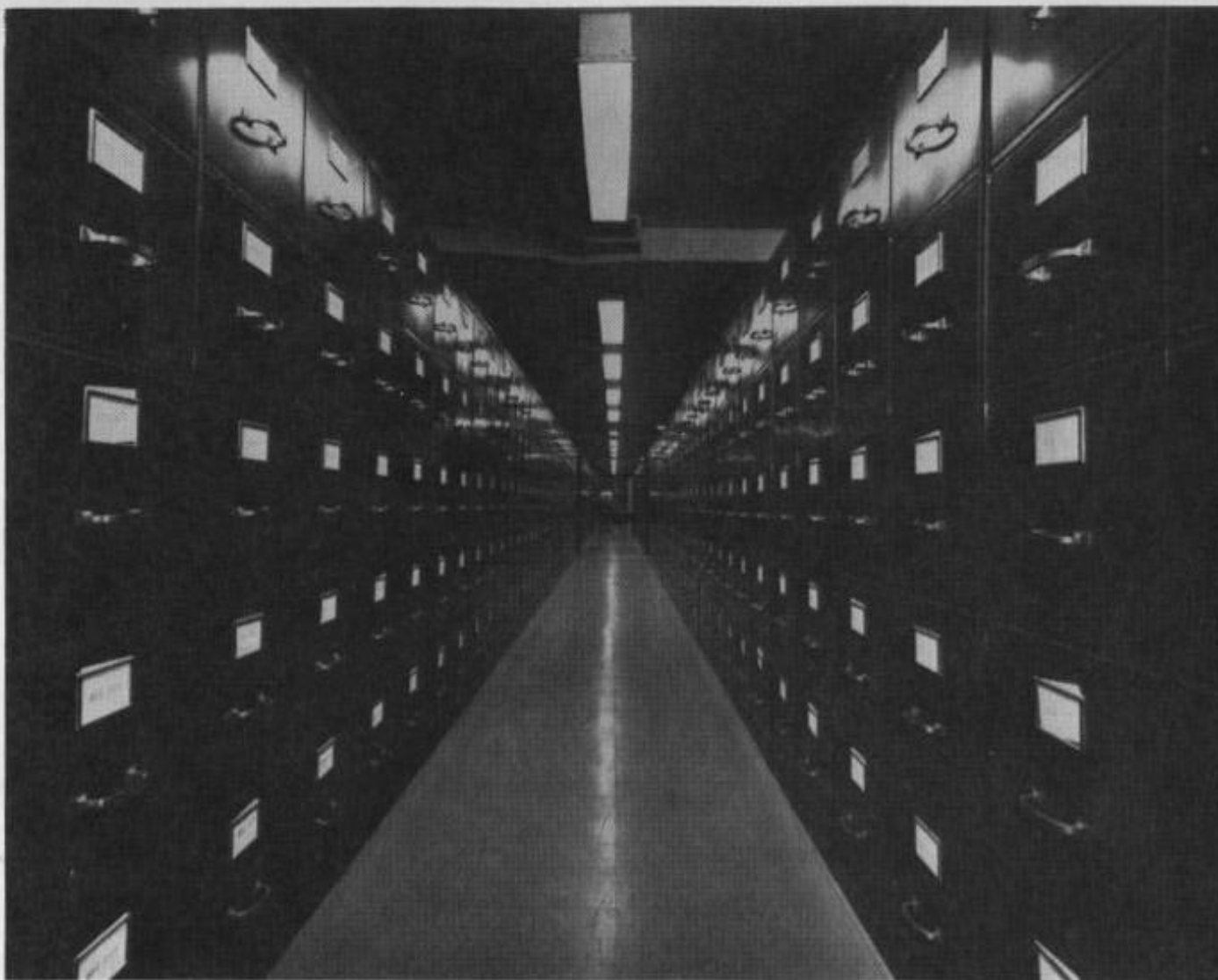
Figure 2.4 Photograph illustrating a vanishing point. Parallel straight lines converge at a single point under perspective projection. This point is called the vanishing point of the straight lines. (Photograph by Herbert Gehr, from the magazine Life , July 1947, © Time Warner, Inc.)
