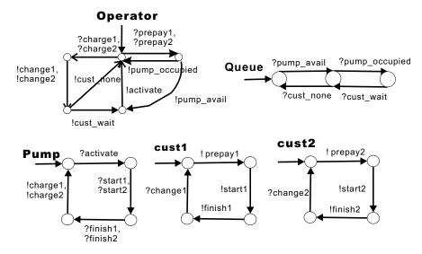
Fig. 7. The state graphs of gas station system
