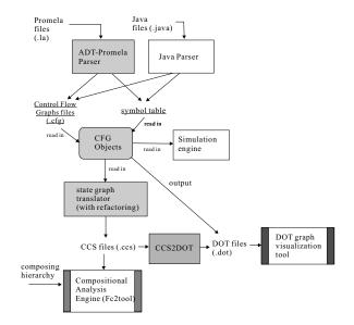
Fig. 8. The framework of tool implementation.
