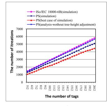
Figure 5. The comparison between PS protocol and ISO/IEC 18000-6B protocol in terms of the number of iterations needed to identify all tags
