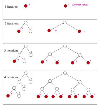
Figure 1. The identification trees of ISO/IEC 18000-6B protocol (left) and PS protocol (right) before the first tag is identified (Note that tag splitting will occur at shaded nodes.)
