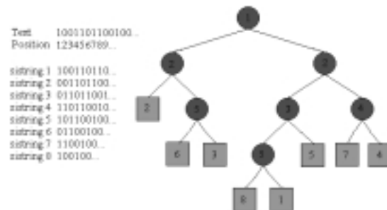
Figure 3: PAT tree when the sistrings 1 through 8 have been inserted
