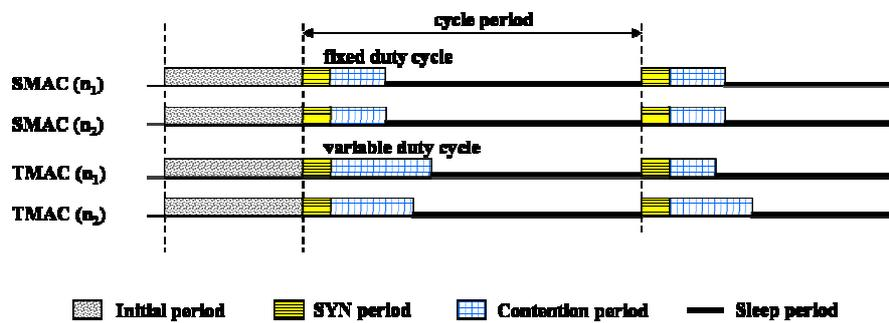
Fig. 2: The duty cycle structures of S-MAC and T-MAC protocols
