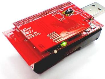
Fig. 6: Octopus II sensor node
