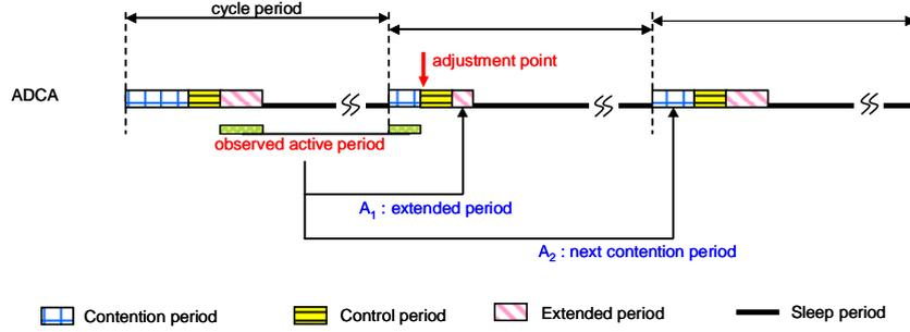
Fig. 4: The duty cycle adjustment of ADCA protocol
