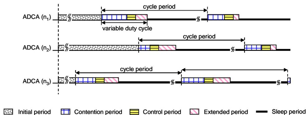
Fig. 3: The duty cycle structure of ADCA protocol
